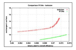
Fig. 2. Rankine cycle optimization- optimal solutions for both R134a and R600a.
