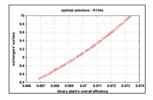
Fig. 1. Rankine cycle optimization - optimal solutions for R134a.
